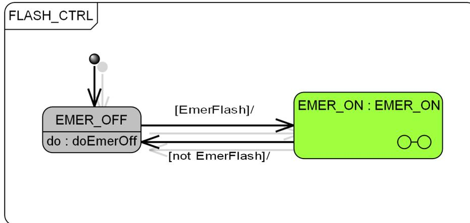
Figure 6: State machine controlling left/right and emergency flashing.
