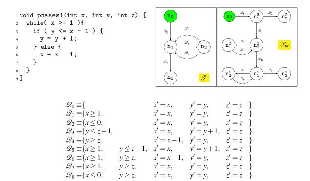
Figure 1: A loop with 2 phases, it corresponding TS  $\mathscr{T}$ , and the TS  $\mathscr{T}_{pe}$  after applying CFR.
