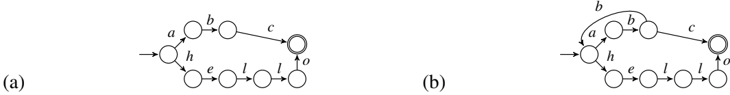
Figure 7: (a) A_1 , \mathcal{L}(A_1) = \{abc, hello\} . (b) A_2 , \mathcal{L}(A_2) = \{abc, hello\} \cup \{(abb)^n c \mid n > 0\} .
