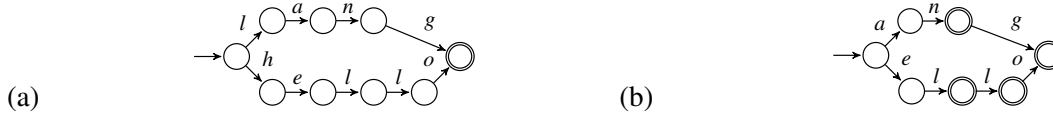
Figure 6: (a) \mathbf{A} , \mathcal{L}(\mathbf{A}) = \{lang, hello\} . (b) \mathbf{A}' = SS^\sharp(\mathbf{A}, [1, 1], [3, +\infty]) , \mathcal{L}(\mathbf{A}') = \{an, ang, el, ell, ello\} .
