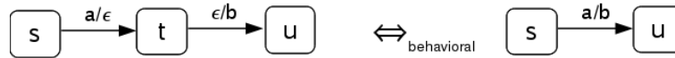
Figure 9: Do the NFIOA on the left and on the right specify the same automaton behavior? In case of a channel based restricted product automaton it depends on what the rest of the automaton is doing.
